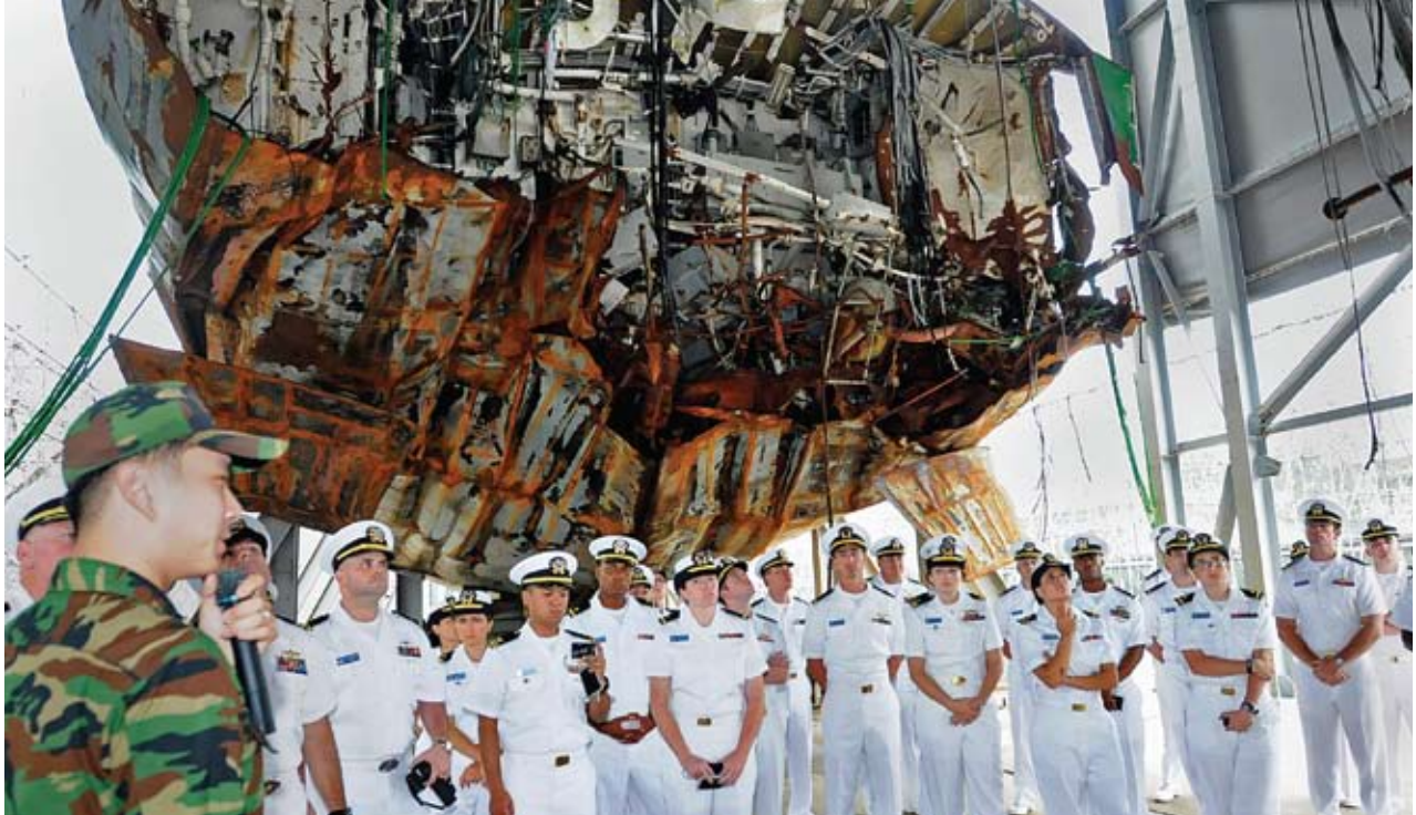
Officers assigned to the U.S. 7th Fleet command ship USS Blue Ridge examine the damage to the Republic of Korea navy corvette ROKS Cheonan . A non-contact homing torpedo exploded near the ship on March 26, 2010, sinking it, and resulting in the death of 46 ROK Navy sailors.
